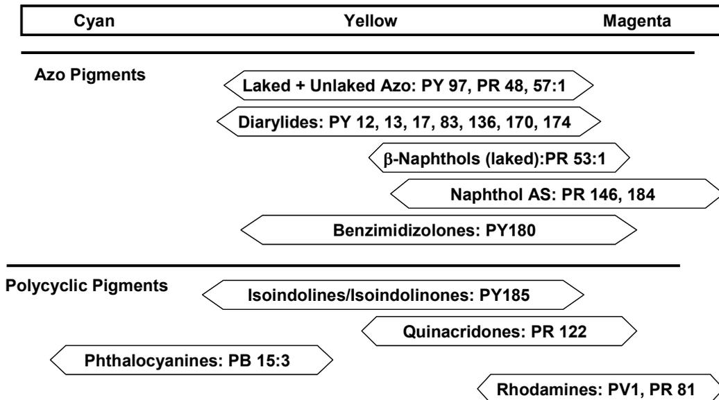
The pigment loading depends upon the color of the toner and hence pigment choice made. Typically the pigment content is from 4 to 20%. For cyan toners the typical choice of pigment is copper phthalocyanine (Pigment Blue 15:3). This
